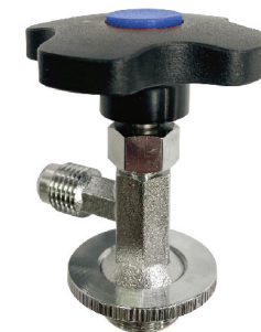
RTM-338: 1/4" SAE outlet valve bottom and female thread fitted with 12mm * 1.25 can thread
