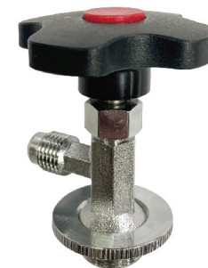
RTM-338: 1/4" SAE outlet valve bottom and female thread fitted with 12mm * 1.25 can thread
